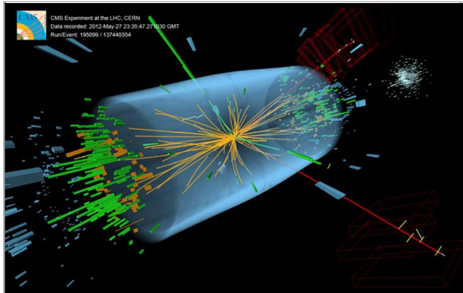
Event recorded with the CMS detector in 2012 at a proton-proton centre-of-mass energy of 8 TeV. The event shows characteristics expected from the decay of the SM Higgs boson to a pair of Z bosons, one of which subsequently decays to a pair of electrons (green lines and green towers) and the other Z decays to a pair of muons (red lines). The event could also be due to known Standard Model background processes.
