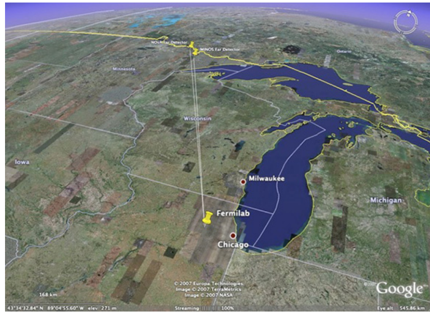
The NOvA project generates a beam of neutrinos from Fermilab to a 15,000-ton detector in Ash River, Minnesota: a 500-mile interstate trip that takes less than three milliseconds {image courtesy of Fermilab}.
